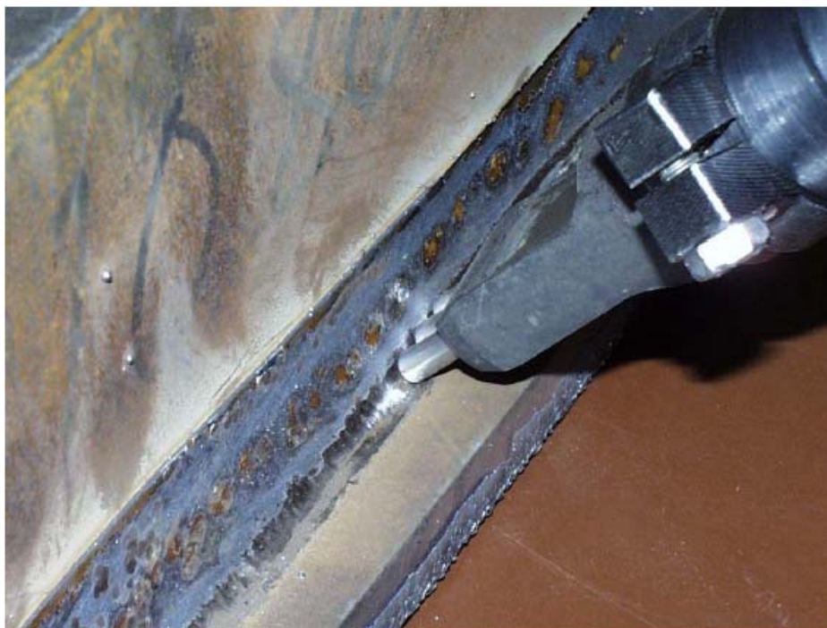
Figure 2. The performance of ultrasonic impact treatment.
