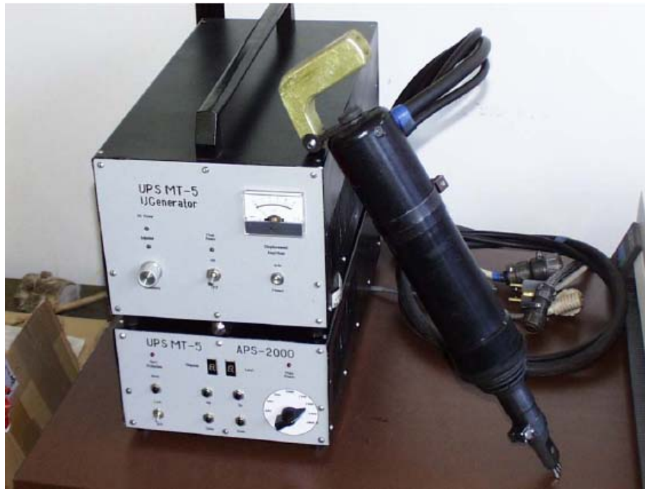
Figure 1. The 27 kHz ultrasonic impact treatment equipment.
